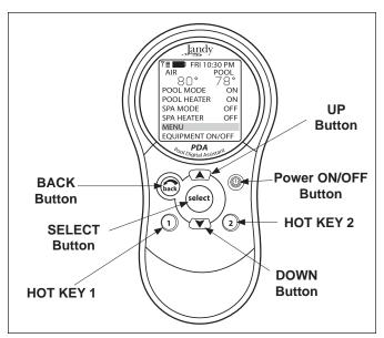
Figure 23. PDA Handheld Remote Buttons
